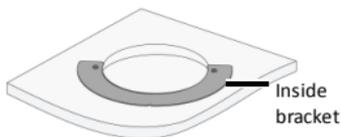
3. Fix the ceiling bracket to the in-ceiling bracket.
