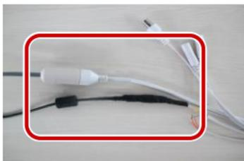
3. Protect other cables using insulating tapes.
