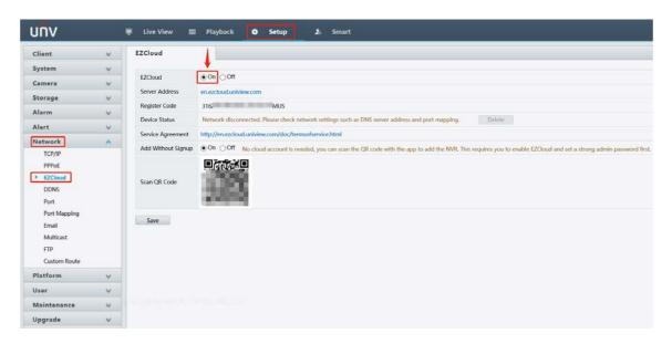
If setting up EZCloud is not an option, you can set up port mapping.
