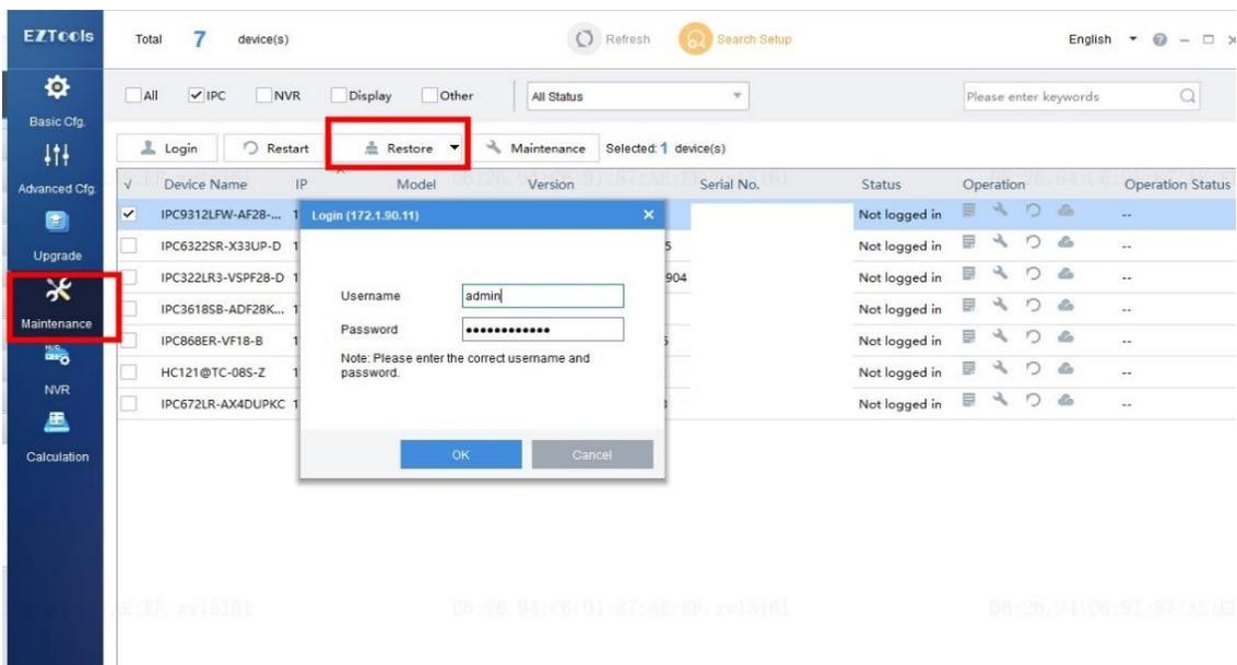
**Note:** Sometimes, the IP address of the camera cannot be found on EZtools even when they are connected to the same LAN. If this happens, please connect the cameras directly to the computer's RJ45 port to see if you can search and find its IP address on EZtools. If you can find the camera, please refer to the steps above.
