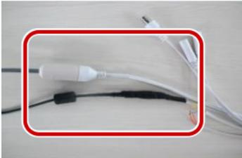
3. Protect other cables using insulating tapes.
